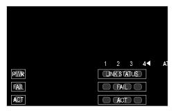
Figure 5-2 Interface Module LEDs
